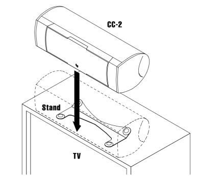
If needed, the enclosed stand allows you to tilt the speaker across a 25-degree range (i.e., 18° up and 7° down), as shown in Figure 3.
